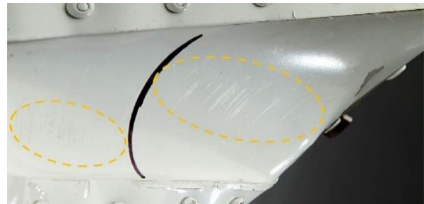
Figure 2. Scratches on aileron rib [13].
