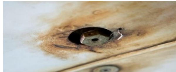
Figure 1. Corrosion on the surface of the aircraft [12].
