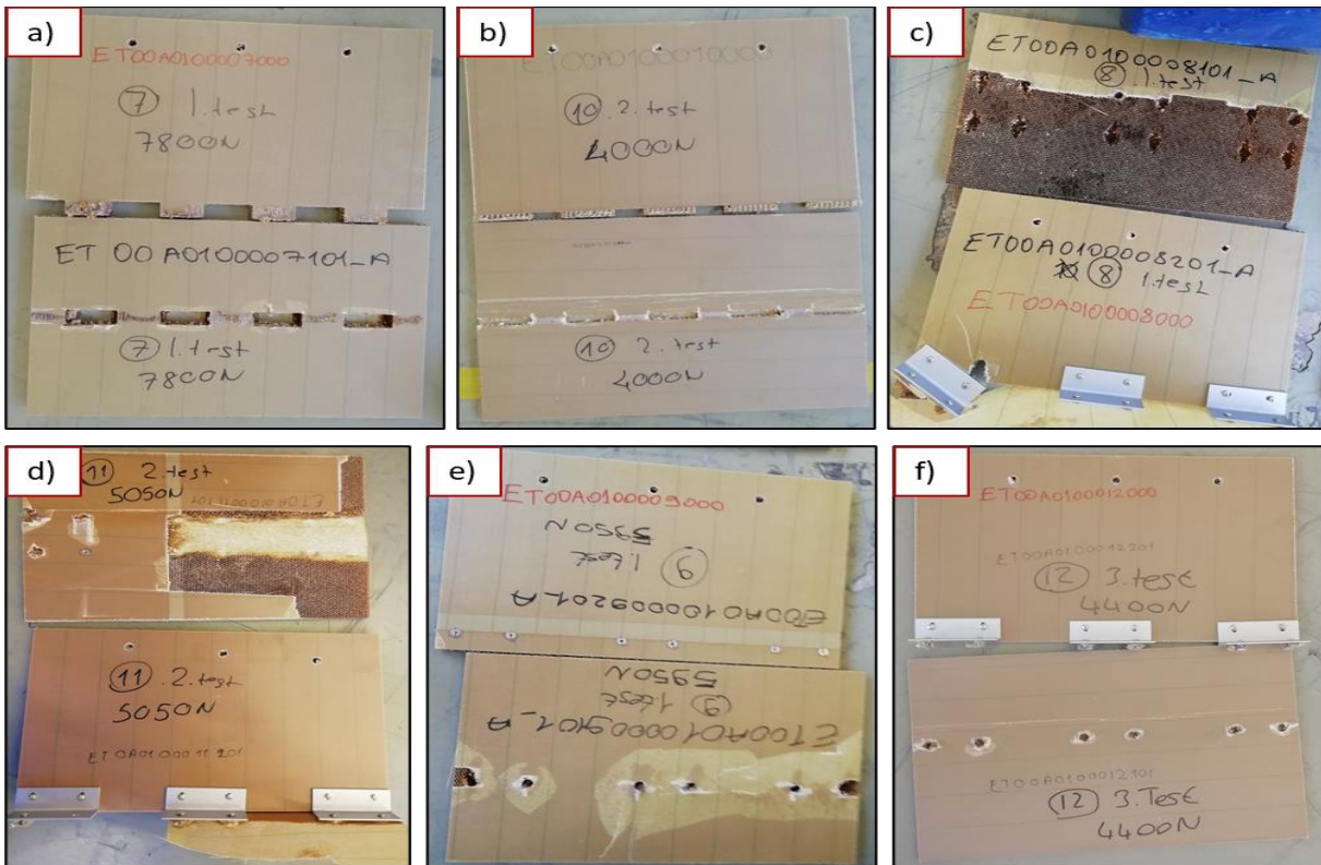
Figure 8. Samples broken as a result of the tensile test: a) 22 mm TM, b) 10 mm TM, c) 22 mm DSB, d) 10 mm DSB, e) 22 mm OSB, f) 10 mm OSB
